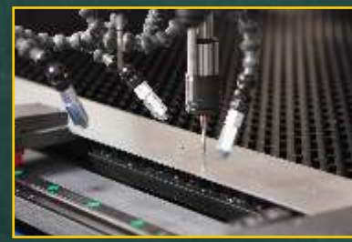
Tapping with air blow lubrication.
