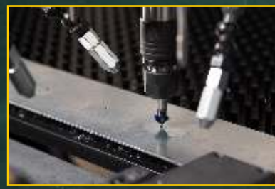
TapOne 1212 with 3 tapping heads up to M10.
